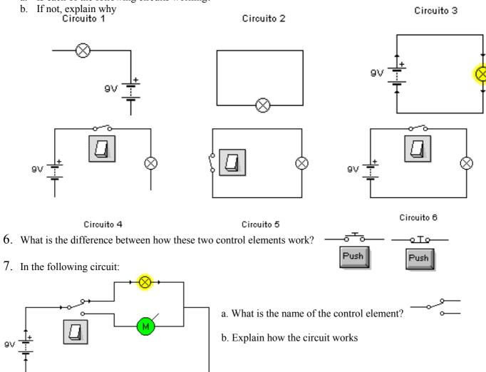
8. In each of the following circuits, explain which control elements are necessary to click/push in order to switch the bulb on.
